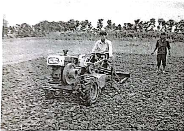
Fig. 2. Field test of power tiller mounted leveler
