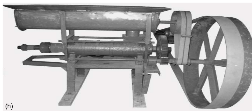
Fig. 1. Different views of the oil expeller: (a) arrangement of agitator in the shaft of the hopper, (b) photographic view of the hopper (c) side view of the shaft of the hopper (d) an worm screw (e) cone of the expeller (f) main shaft of the expeller (g) assembly of the screws in the crushing chamber and (h) assembly of the whole expeller and frame for setup.
