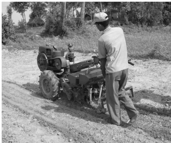
Photo 1. Planter in operation for seeding sprouted seed
