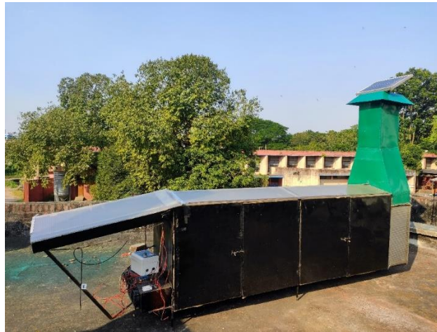
Figure 3. BAU Solar Chimney Dryer with modified auxiliary heating system
