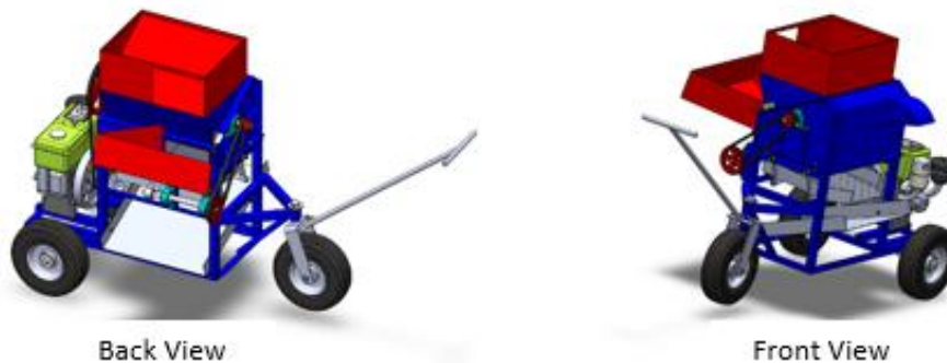
Figure 2. Orthographic views of the sunflower thresher
