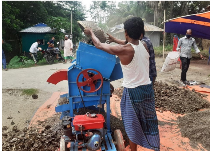
Figure 5. Operational view of the power sunflower thresher at Subarnachar Noakhali
