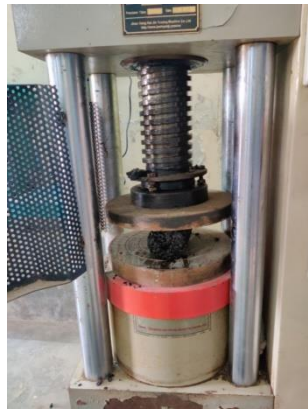
Figure 6. Split tensile strength test of sample
