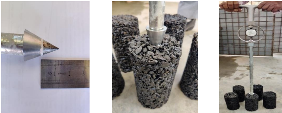
Figure 5. Penetration test of sample
