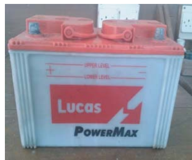
12V DC storage battery
