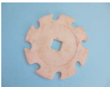
Fig. 2: A photographic view of a seed metering device
