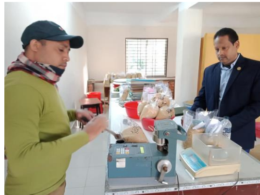
(b) Measurement of moisture content of stored paddy
